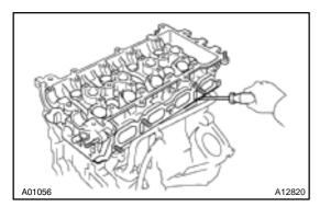
(d) Using a screwdriver, pry between the cylinder head and cylinder block, and remove the cylinder head.NOTICE:
