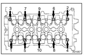
(b) Using a 10 mm bi–hexagon wrench, uniformly loosen and remove the 10 cylinder head bolts in several passes, in the sequence shown.
